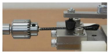
Anchor the metal cap to the temple tip at two points as shown in the picture. And pull from the temple tip part and measure the strength.
