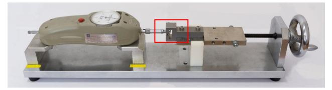
Measure tensile strength of a ceramic nose pad using the Pulling Tester as shown in the picture.
